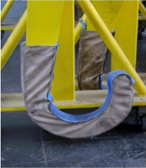
Photo 2 : Lifting device of crane for wheelsets with axles boxes, release protective
