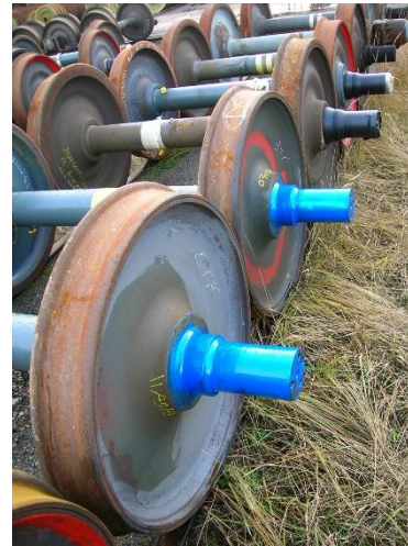
Photo 8: wheelsets storage without axles boxes (running gear protected by paint)
