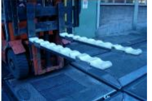
Photo 8: Wheelset holder for fork-lift truck (several wheelsets)
