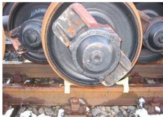
Photo 2: Storing in staggered formation on track using safety scotches
