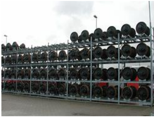
Photo 5: Stacking of wheelsets in loading cradles
