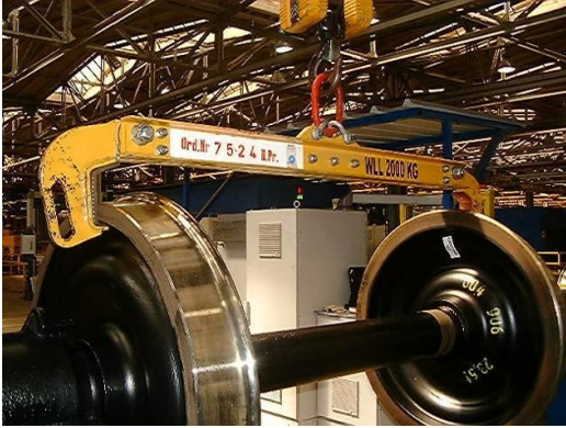
Photo 4: Wheelset holder for fork-lift truck
