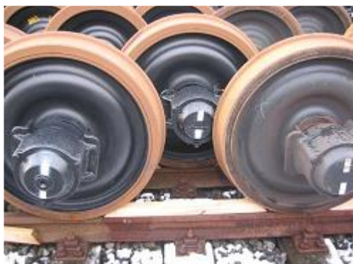
Photo 3: Storing in staggered formation (with double rail)
