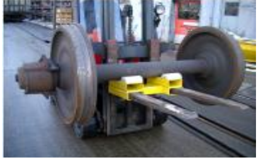
Photo 7: Wheelset holder for fork-lift truck (loaded)
