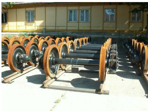
Photo 1: Storing on track using safety scotches
