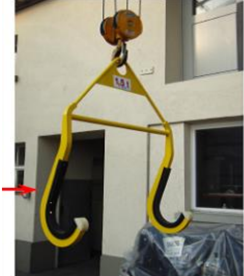
Photo 1: Lifting device of crane for wheelsets with axles boxes (axle shaft.)
