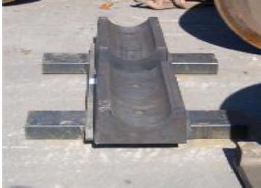
Photo 5: Wheelset holder for fork-lift truck
