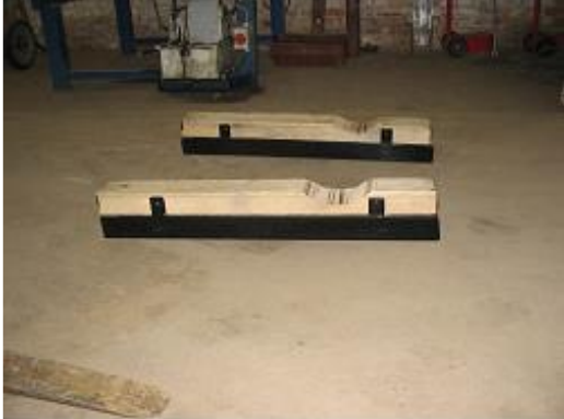
Photo 6: Wheelset holder for fork-lift truck
