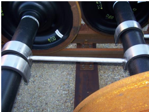
Photo 7: Storing in staggered formation (with double rail) with spacers
