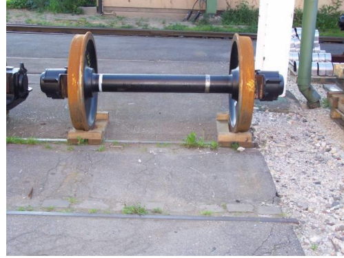
Photo 6: individual storage using lockers storage for single axles
