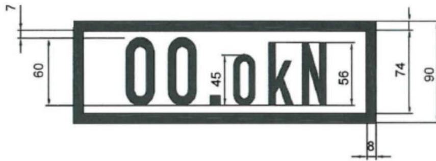
Figure 4: Marking indicating the holding force in kN on wagons fitted with screw brakes.
