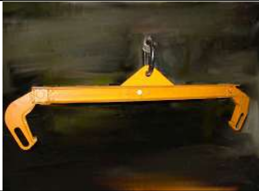
Photo 3: Lifting device of crane for wheelsets (wheel disc)
