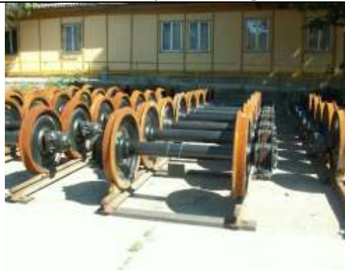
Photo 1: Storing on track using safety scotches
