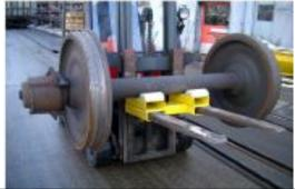
Photo 7: Wheelset holder for fork-lift truck (loaded)
