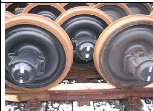
Photo 3: Storing in staggered formation (with double rail)
