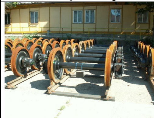
Photo 1: Storing on track using safety scotches
