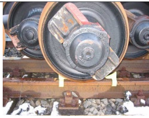
Photo 2: Storing in staggered formation on track using safety scotches
