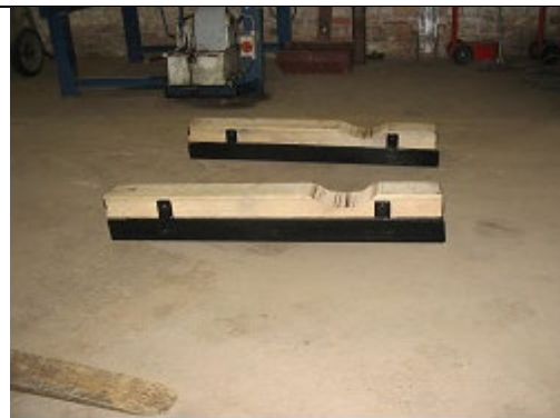
Photo 6: Wheelset holder for fork-lift truck
