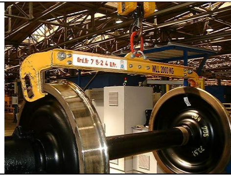
Photo 4: Wheelset holder for fork-lift truck
