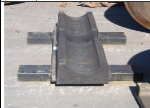
Photo 5: Wheelset holder for fork-lift truck
