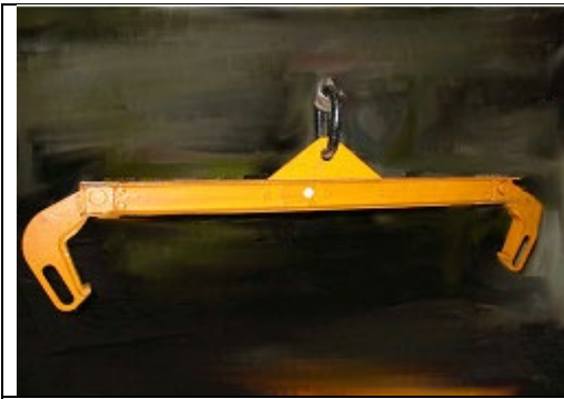
Photo 3: Lifting device of crane for wheelsets (wheel disc)
