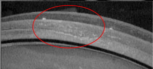
Picture 8: Irregular contact surface on the edge of tyred wheel rim
