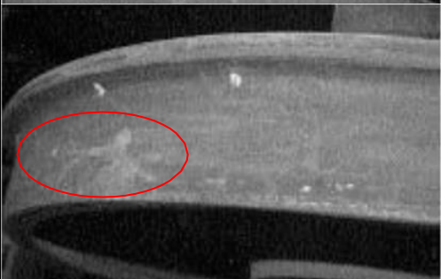
Picture 9: Major irregular crushing of the edge of the tyred wheel rim
