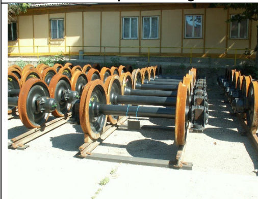
Photo 1: Storing on track using safety scotches
