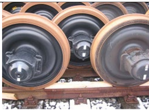
Photo 3: Storing in staggered formation (with double rail)
