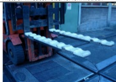
Photo 8: Wheelset holder for fork-lift truck (several wheelsets)
