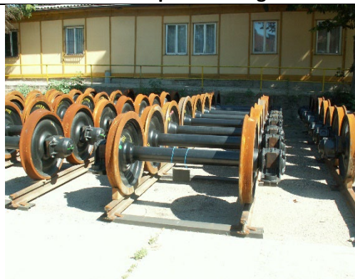
Photo 1: Storing on track using safety scotches
