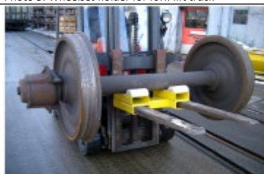
Photo 7: Wheelset holder for fork-lift truck (loaded)
