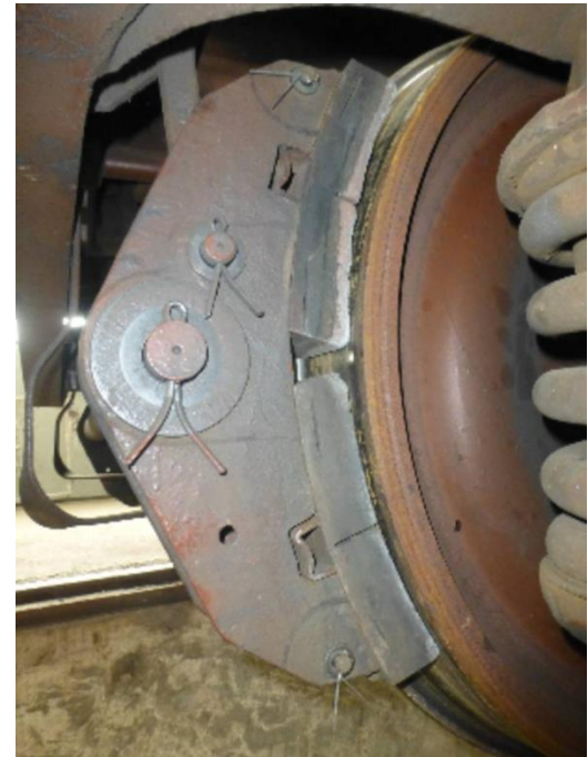
Melted brake block
